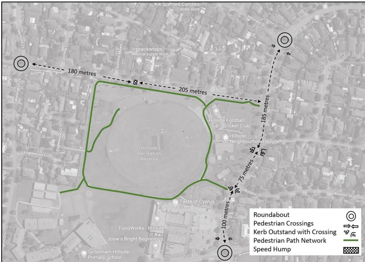
Figure 4 shows distances of less than 200 metres between LATM devices. This falls below the threshold for consideration of further traffic calming measures outlined in Council’s Traffic Calming Policy.
