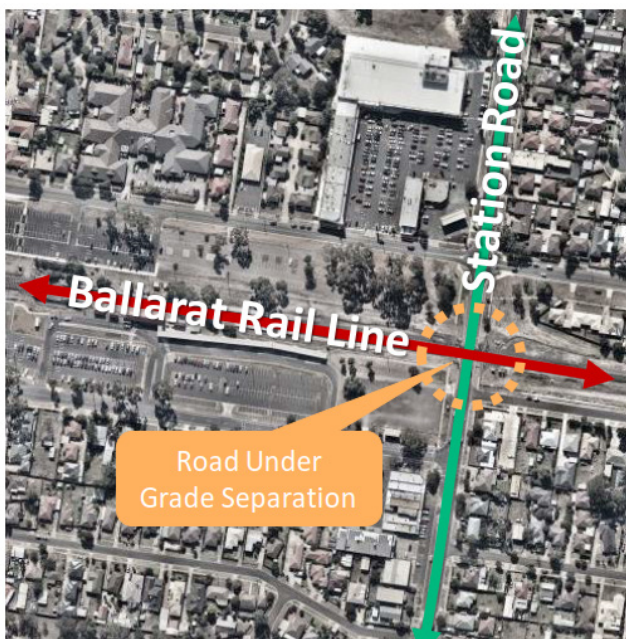
Fig. 50 Road under grade separation diagram.
