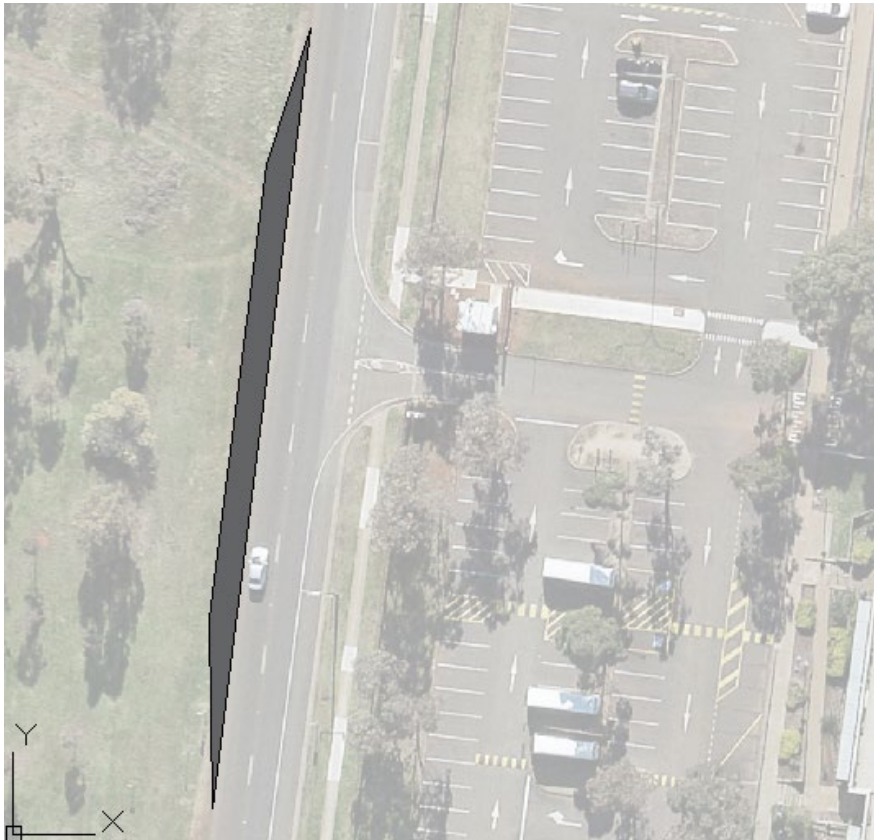
Figure 4 Basic Auxiliary Right (BAR) treatment at north access
