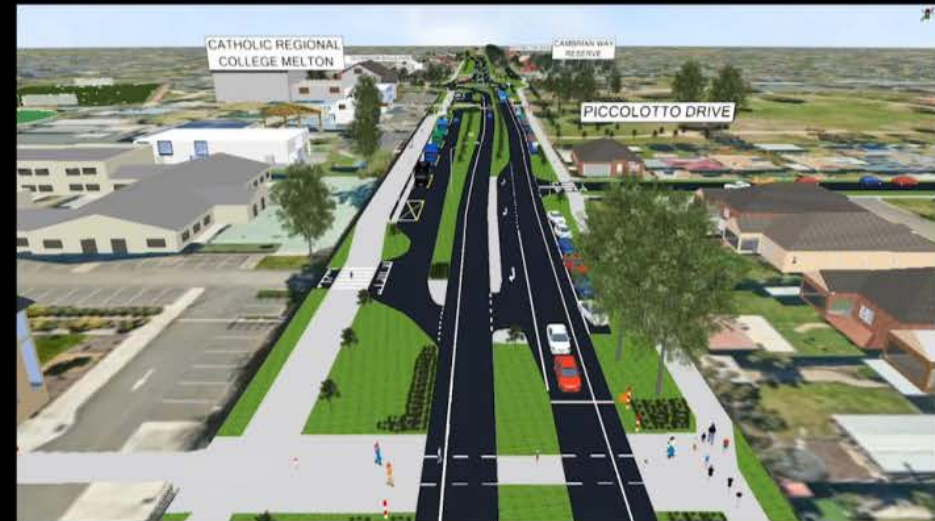
SAFER INTERSECTION & SEPERATE TURNING LANES
