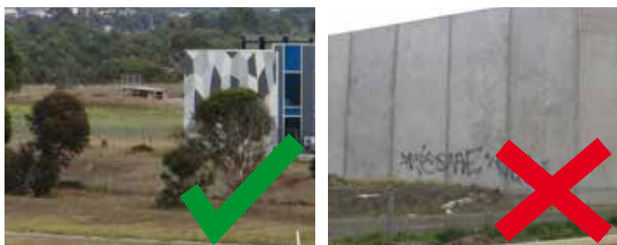
Figure 72 - Uses should address a freeway frontage rather than creating a blank and graffiti-prone interface
