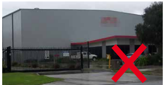
Figures 26 and 27 - Offices should be a minimum of 40% of the main building height to minimise the visual bulk of industrial building facades
