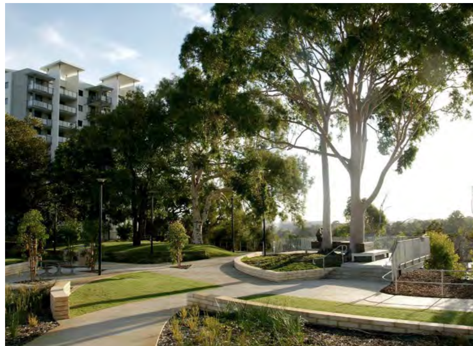
A mixture of hard and soft landscaping elements is appropriate for an urban park, as it enables year-round use
