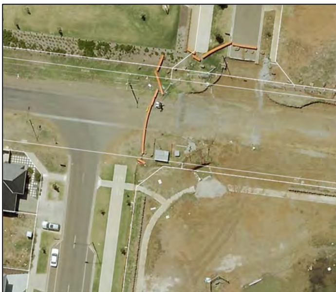
Example of a Full Road Closure
