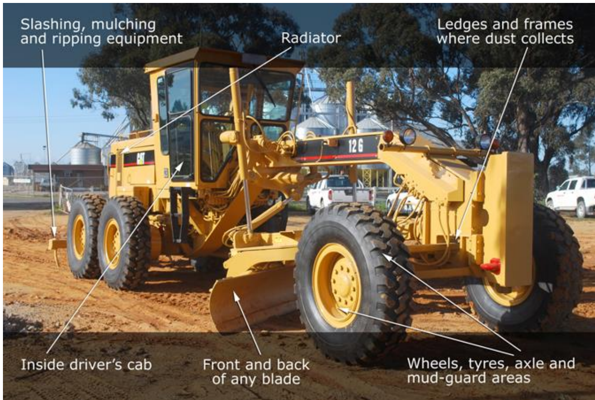
Figure 10: Machinery washdown checklist. Source: EPA Victoria.
