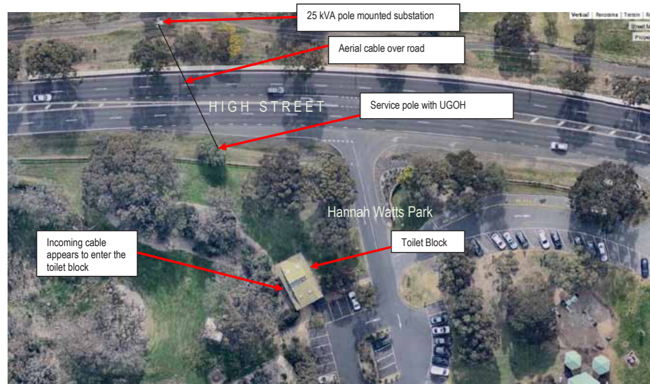
Fig 3 Plan view of power supply to site
