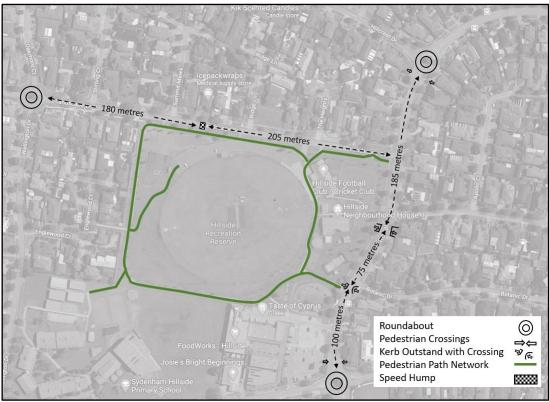
Figure 4 shows distances of less than 200 metres between LATM devices. This falls below the threshold for consideration of further traffic calming measures outlined in Council's Traffic Calming Policy.
