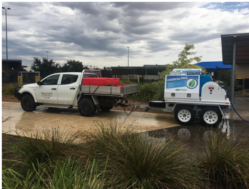
Fig 1: Steam Weeding Unit at Springside, Caroline Springs.
