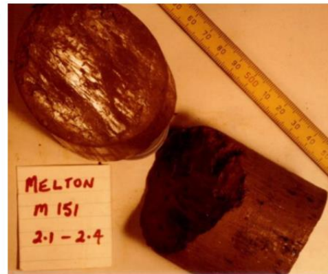
Figure 5. Polished shear surface, or slickenside, in a clay core sample from Melton Sourced from: (Dahlhaus, 1986d; 1988)
