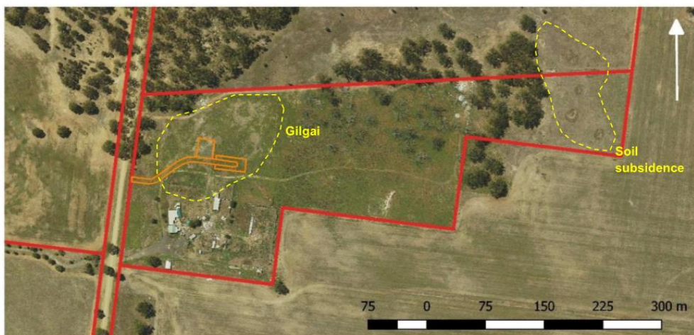
Figure 14. Some of the more obvious geohazards at the proposed development site as seen in aerial imagery. (source Melton City Council. Imagery captured January 16, 2018)
