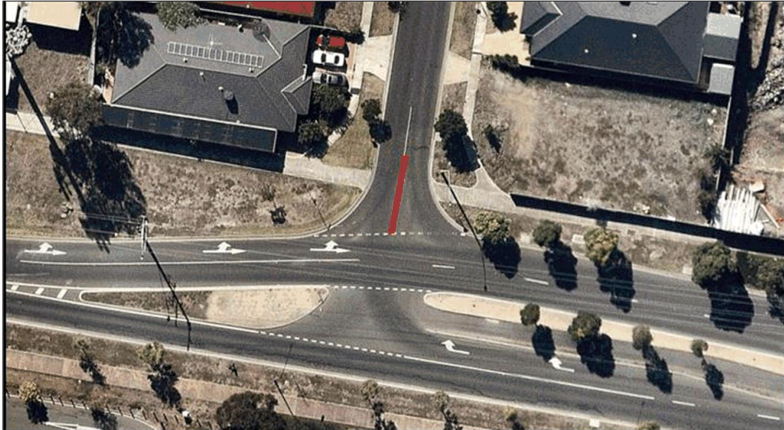
Figure 18 Conrad Terrace / Taylors Road – Splitter Island
