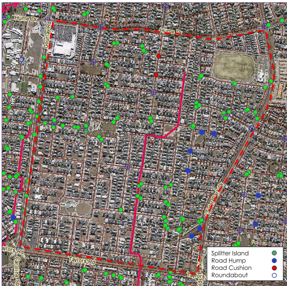
Figure 5 Existing LATM Treatments
